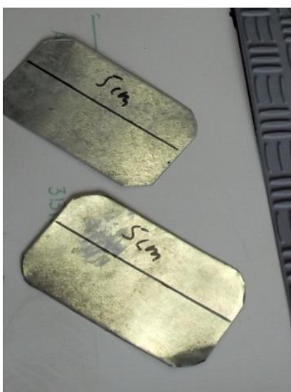
Image 02: Prepare two sheets of metal, approx. 20 cm x 12 cm, e.g., made of galvanized sheet metal. Mark lines parallel to the long edge at intervals of 5 cm..
